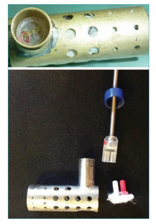
Figure 2. The PinPort<sup>™</sup> tail cuff in-situ during the recirculation phase.
