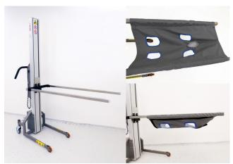
To have an alternative we fitted an industrial lift with forks that can carry the slings. The forks can be lowered to the ground to have the option to train the Göttingen Minipigs to step into he sling by itself and to be raised to a comfortable working position
