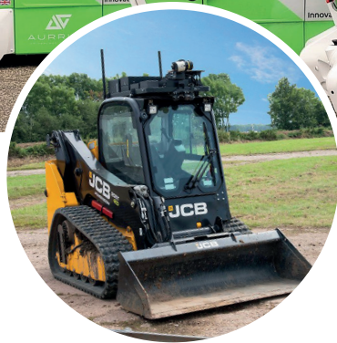
◀ UK manufacturers such as JCB are leading the way in the development of automated industrial vehicles, such as this driverless JCB Compact Track Loader
